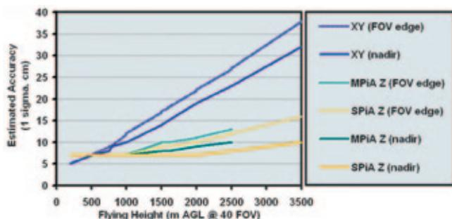
Leica ALS70-CM and ALS70-HP provide high accuracy, even in MPiA mode
