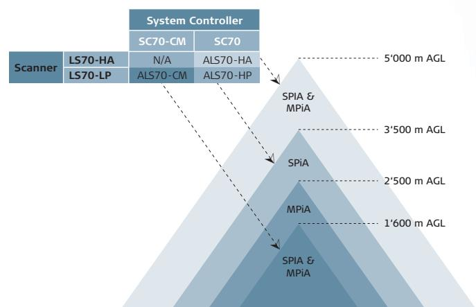
**Leica ALS70-CM** is designed for city and corridor mapping applications from lower flying heights. Ultra-high-density can be achieved by flying in small aircraft or mounted in helicopter pods, taking advantage of the low-profile scanner.
