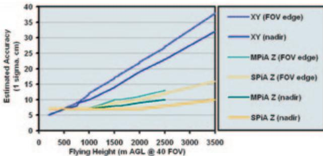
Leica ALS70-CM and ALS70-HP provide high accuracy, even in MPIA mode
