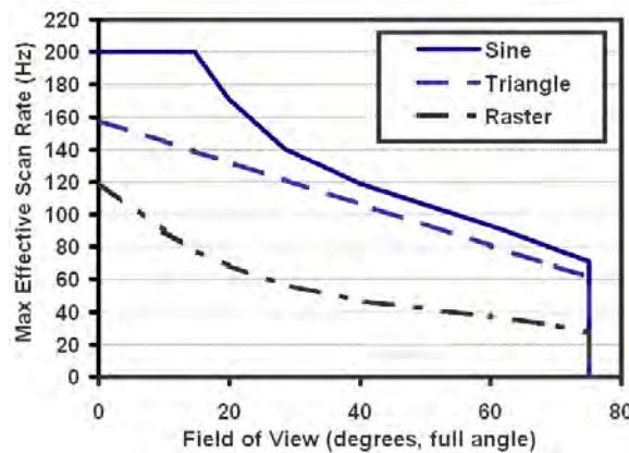
The scan rate is user-selectable from 0 to 200 Hz (depending on scan pattern selected) in 0.1 Hz increments via the graphical user interface. System control software prevents out-of-range inputs for scan rate based on user selection for FOV and scan pattern.
